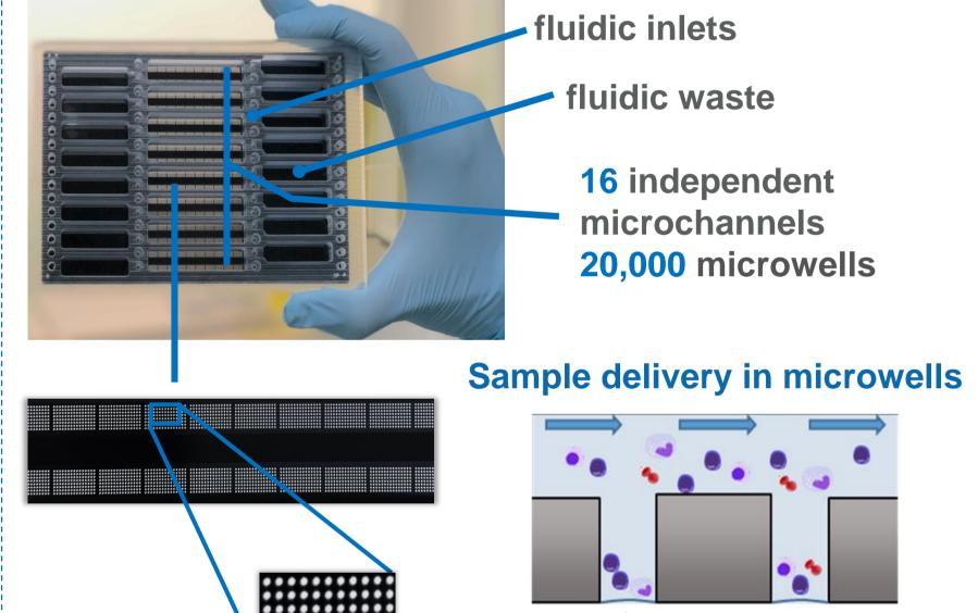
The Open Microwell (OMW) is a microfluidic device on which living cells extracted from ex-vivo patient samples are loaded through an automatic liquid handling system, forming 20,000 miniaturized heterogeneous cell clusters in microwells and allowing analysis of cell-cell interactions in each cluster under the action of specific treatments. Each of the 16 independent microchannels is used to test a different condition (e.g. a drug at a specific dose) on a group of 1,200 microwells.
